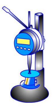
A Digital Thickness Tester is used to measure the gauge or thickness of a fabric which is directly correlated to fabric insulative properties, porosity, as well as a fabric's capacity to drape over a three dimensional form. The measure of fabric thickness is an essential element of a fabric's usefulness in product form.
